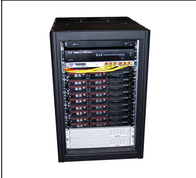
Figure 10: an example of small cluster supercomputer, made by 8 chassis each contain a “computational node” made of 2 AMD Opteron 242 CPUs sharing a memory module of 1 GiBytes. Each computational node is a small SMP and is interconnected with the other by a dedicated 1 Gigabit internal network. This hybrid cluster computer is installed at the Bioinformatics and High Performance Computing Lab of the Bioindustry Park of Canavese ( http://www.bioindustrypark.it/ ).
