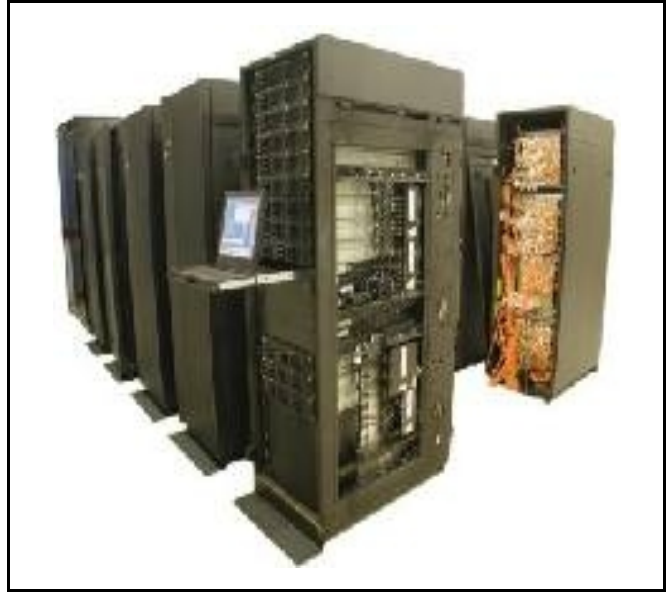
Figure 11: an example of a large scale cluster supercomputer installed at Cineca. It is an IBM Linux Cluster 1350 made of 512 IBM X335 computational nodes. Each computing node contains 2 Xeon Pentium IV CPUs that share together 2 GiBytes of work memory. Each black “armchair”, also called rack, contains many chassis, each chassis contains a certain number of computational nodes.
